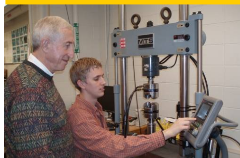
Prof. Y. Kin and student conducts a fatigue experiment
